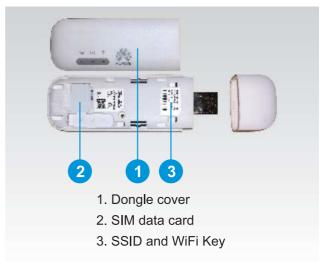
Remove the WiFi dongle cover and insert an activated data card. The Ogauge has been fed with the SSID and WiFi key of this dongle. Please use this dongle with your laptop, when demonstrating the dashboard to the client.
